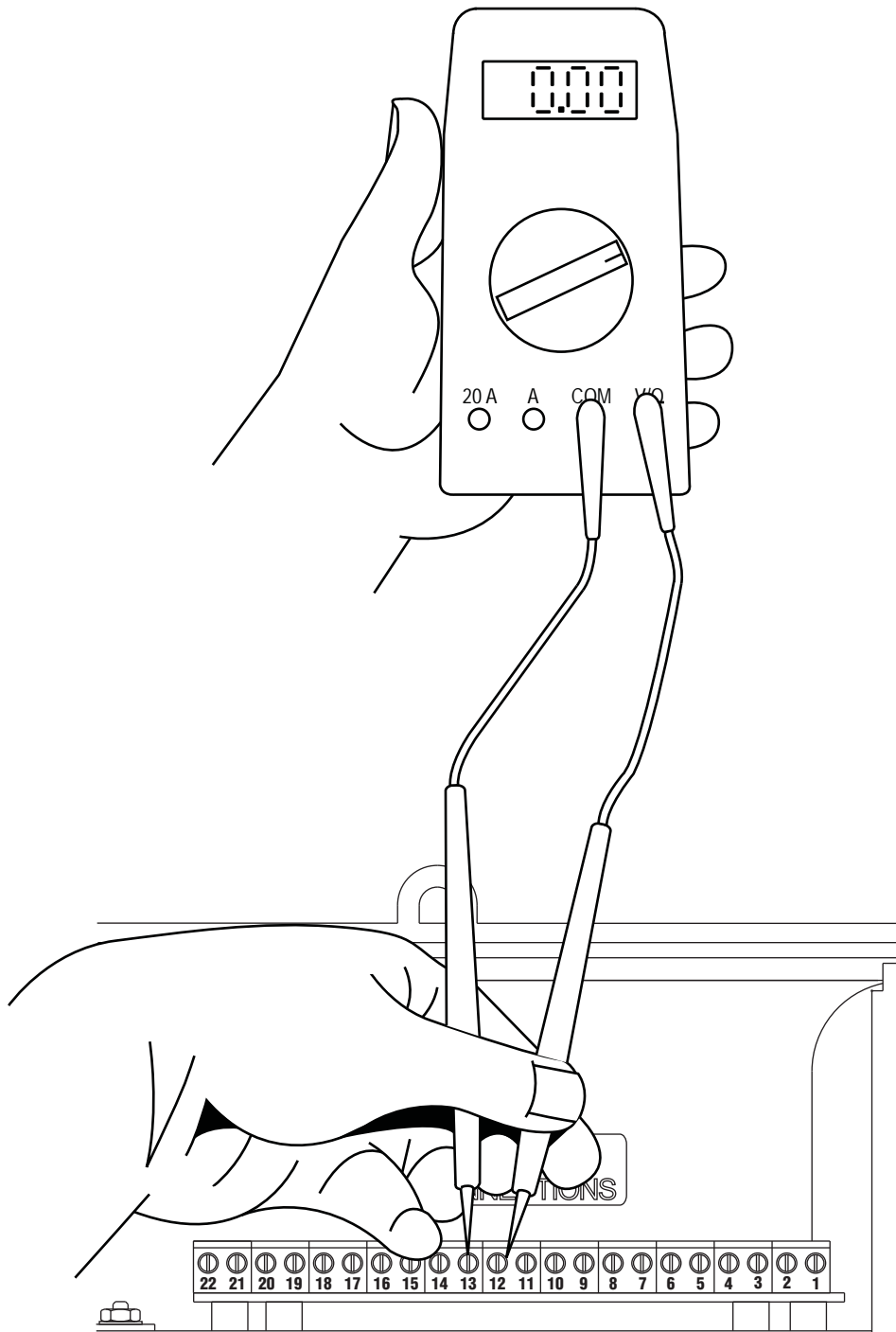
Figure 21: APS-3C/APS-4C/SC-40C Electrician's DVM Connection Between Pins 12 and 13.
